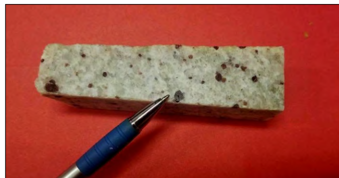
A peraluminous granitoid sample with subhedral garnet that was donated to the Department of Earth Sciences, UNB by Dr. Barrie Clarke. The sample is from India with the commercial name of "Kashmir White Granite".
