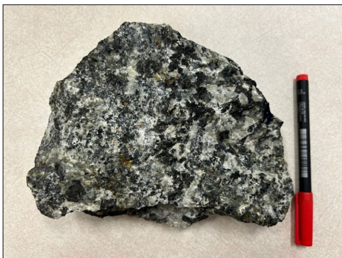
Figure 7: Gabbroic sample from Marathon Cu-PGE sulfide deposit with bornite ( \text{Cu}_5\text{FeS}_4 ) and chalcopyrite ( \text{CuFeS}_2 ).
